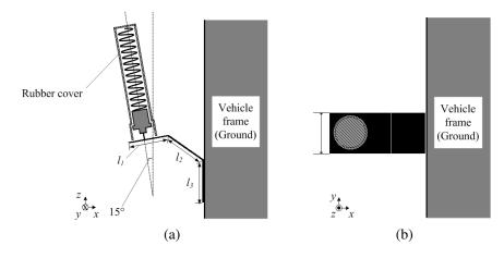
Figure 5. Geometry of the antenna mounted on the frame. (a) Side view. (b) Top view.
