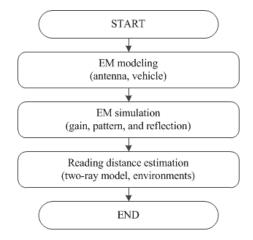
Figure 1. Flow chart of the estimation method for vehicular RKE antennas.
