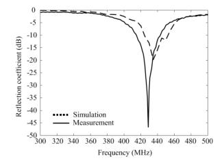
Figure 6. Simulated and measured reflection coefficients.
