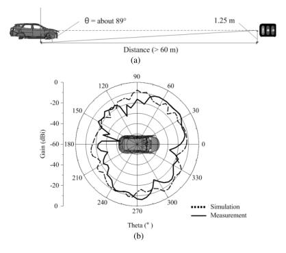
**Figure 7.** Simulation conditions and results. (a) Simulation conditions of the radiation pattern. (b) Simulated and measured radiation patterns at 434 MHz.
