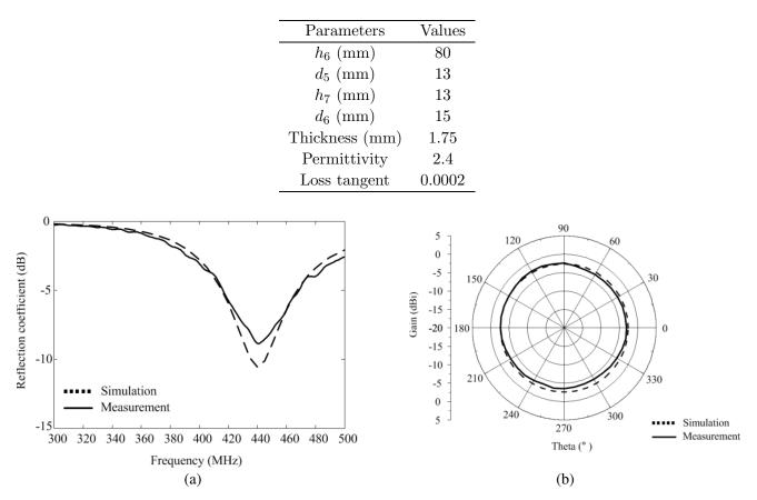
Figure 3. Simulated and measured results. (a) Reflection coefficient. (b) Azimuth radiation pattern at 440 MHz.
